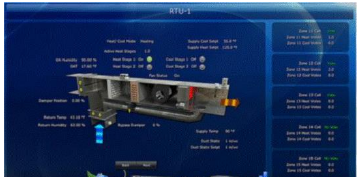
Web Based Building Automation Interface
