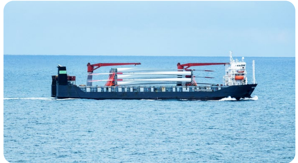
Figure 2-43. WTG blades being transported to marshaling harbor.
