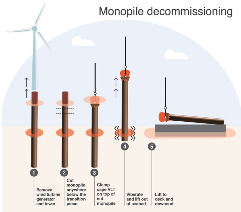
Figure 16-4. Full monopile removal process using vibratory technology (Image adapted from CAPE Holland; for illustrative purposes only).
