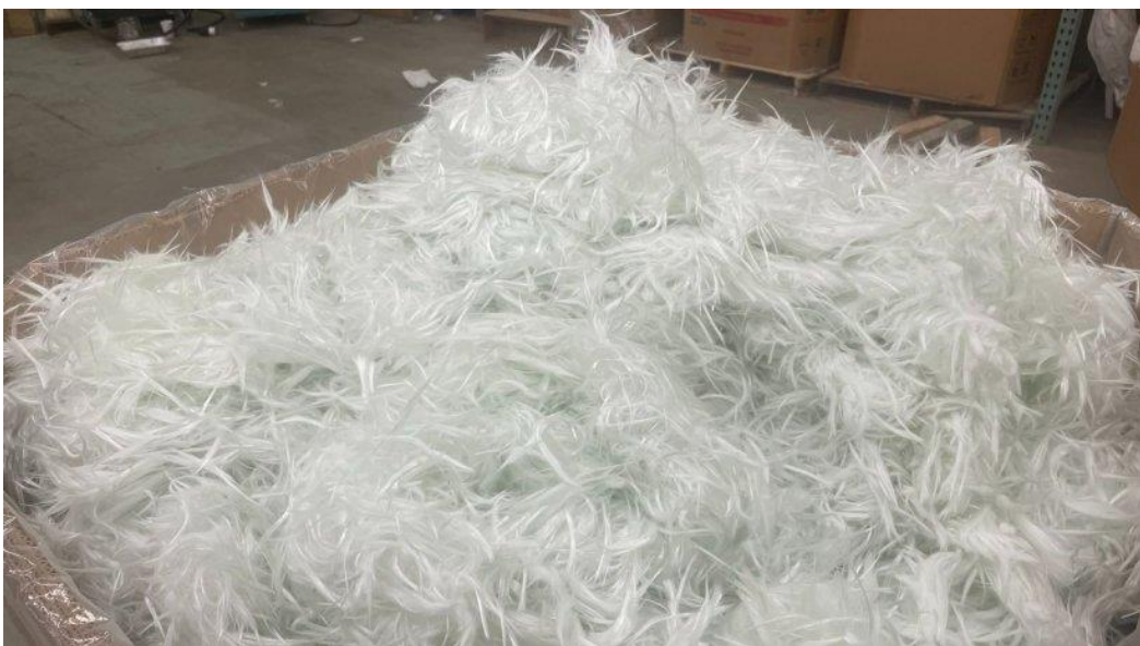
Figure 5-1: Recycled glass fiber from Carbon Rivers (source: US Department of Energy).
