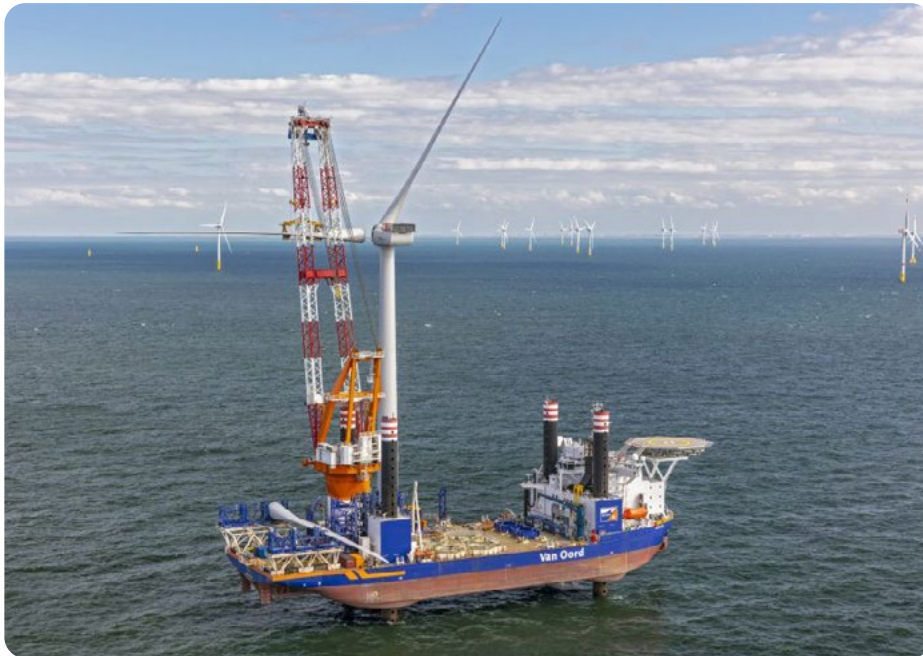
Figure 10.1-2. Wind turbine installation vessel. Courtesy of Van Oord.
