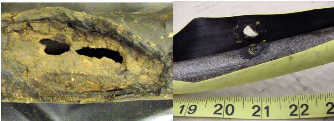
**Figure 11. Puget Sound Energy - Coated Steel Services – Corrosion and Leak**
