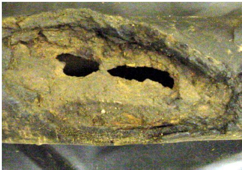
**Figure 35: PSE Spirit Ridge Service Failure-External Corrosion**
