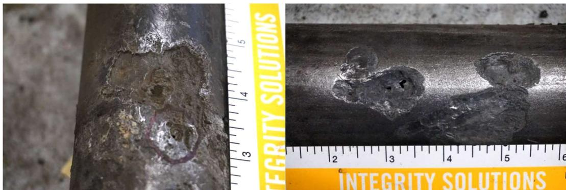
**Figure 12. South Jersey Gas - Steel Mains - Corrosion Leaks**
