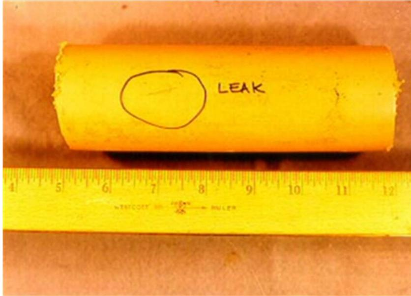
**Figure 13: Slit Fracture on Plastic Pipe Manufactured by DuPont**
