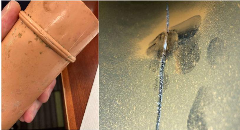
**Figure 15: ETG Plastic Pipe Leaks at Joint and Split**
