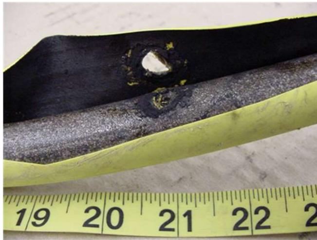
**Figure 37: Photograph of Coating Holiday and Corrosion Damage (PSE)**
