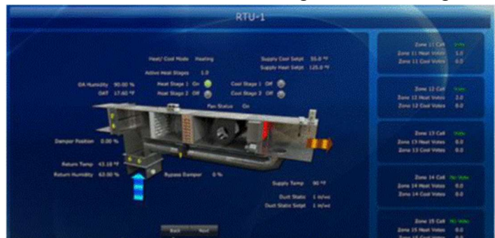
Web Based Building Automation Interface
