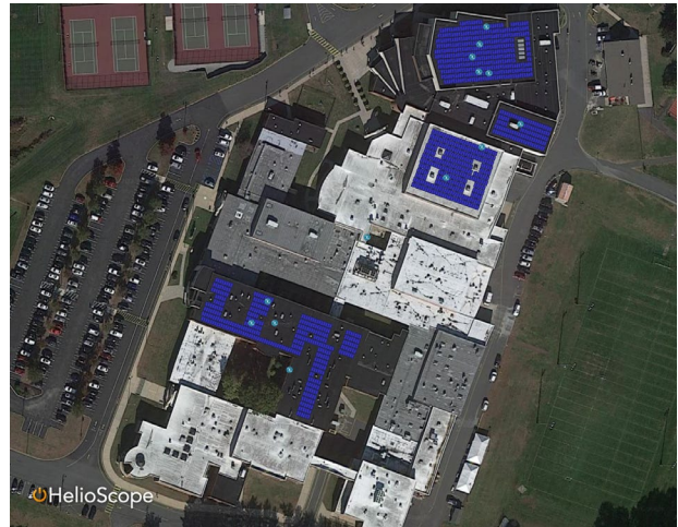
Potential Rooftop Solar Array at Clearview HS
