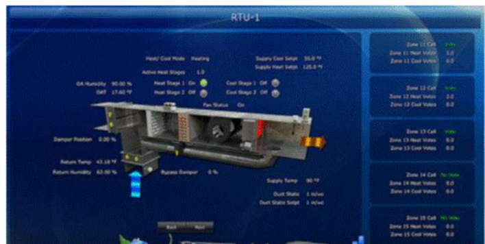
Web Based Building Automation Interface
