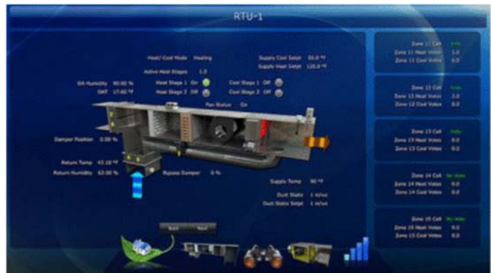
Web Based Building Automation Interface
