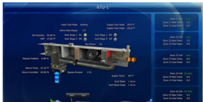
Web Based Building Automation Interface
