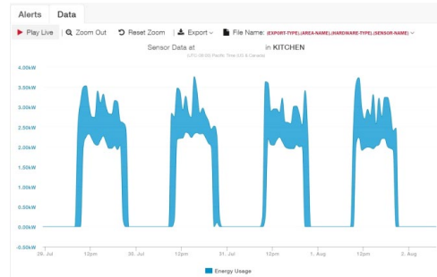
Figure 3. Locking Out Kitchen Exhaust Saves Energy
