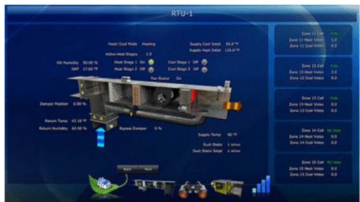
Web Based Building Automation Interface
