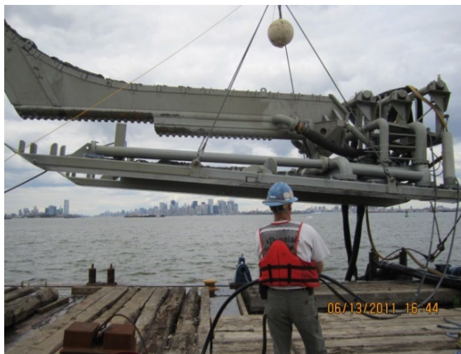
Graphic 4. Typical Jet Plow used for Submarine Cable Burial
