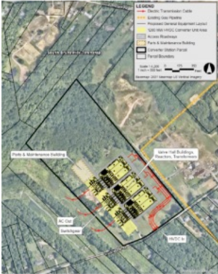
One of three 1200 MW onshore converter stations
